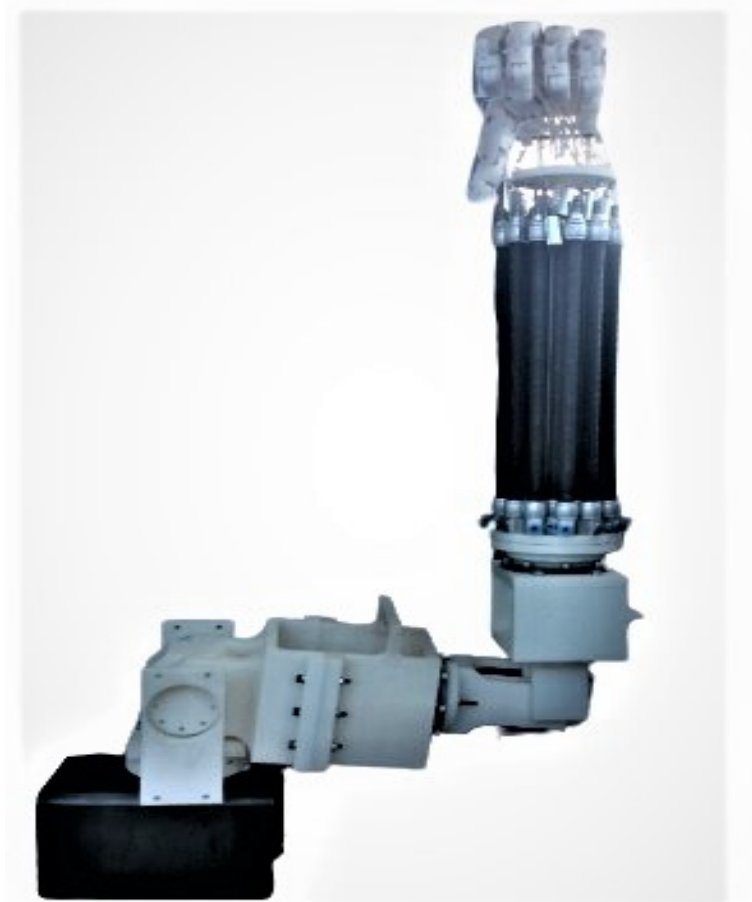
Figure 3.18: The ambidextrous robot arm in its default position.
