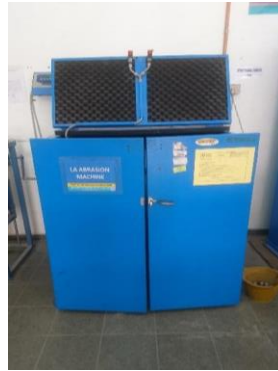
Figure 2. Los Angeles Abrasion Machine
