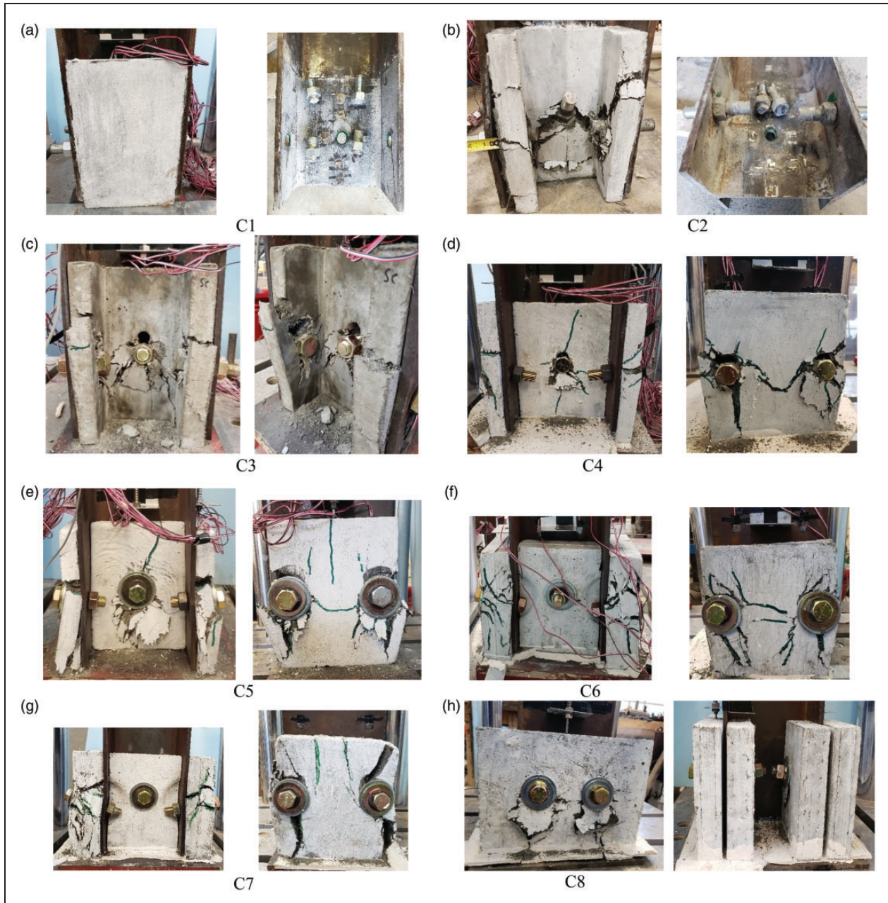
Figure 5. Failure modes of the test specimens: (a) C1, (b) C2, (c) C3, (d) C4, (e) C5, (f) C6, (g) C7, and (h) C8.
