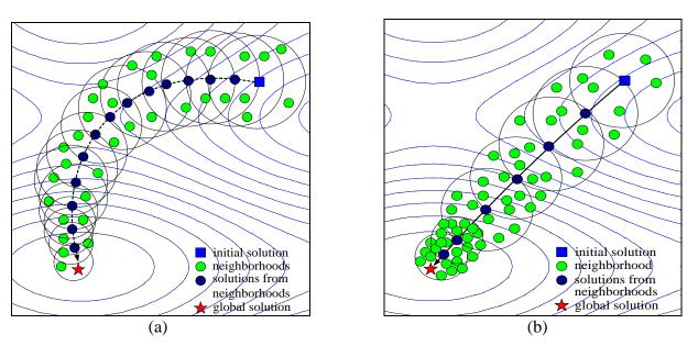
**Fig. 2** Effect of number of neighborhoods to the straightforward direction to the global solution (a) ATS, N=3 and (b) mATS, N=5 (for example).
