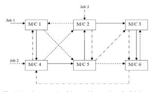
**Fig. 1.** Another example of the machine routings for 3-jobs 6-machines scheduling problem.
