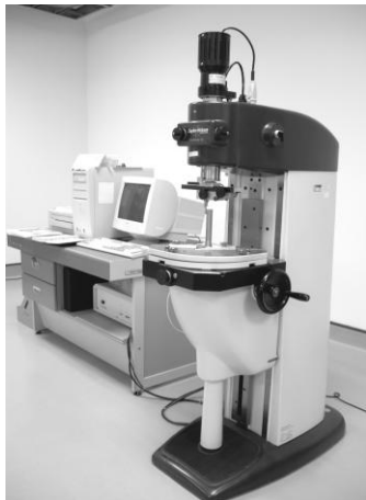
Fig. 1. Roundness measuring instrument, Talyrond 73.
