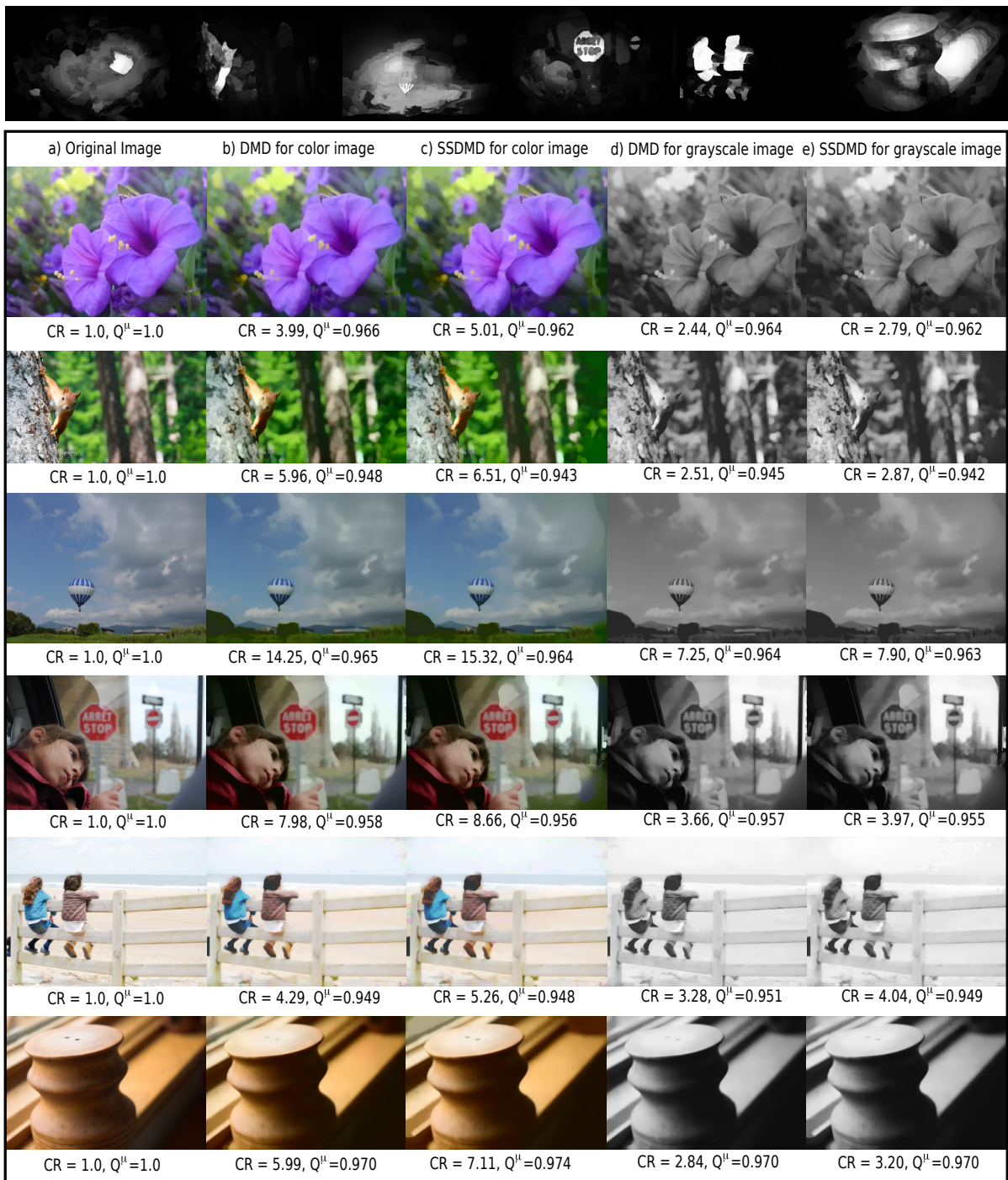
Figure 6: Comparison of the DMD with the SSDMD method for color and grayscale versions of six input images. The top row shows the spatial saliency maps of each input image. For each image, we show the compression ratio CR and quality score Q^H .
