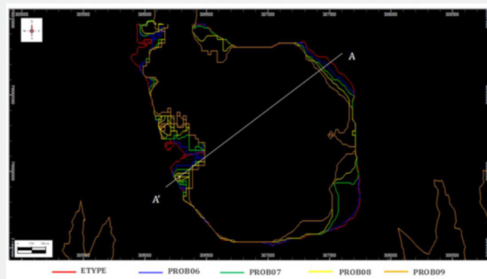
Figure 4: Plan view at the 1230 m level of the final pits for each risk scenario, taking account of the simulated block model associated with the probabilities shown by the differently colored lines.
