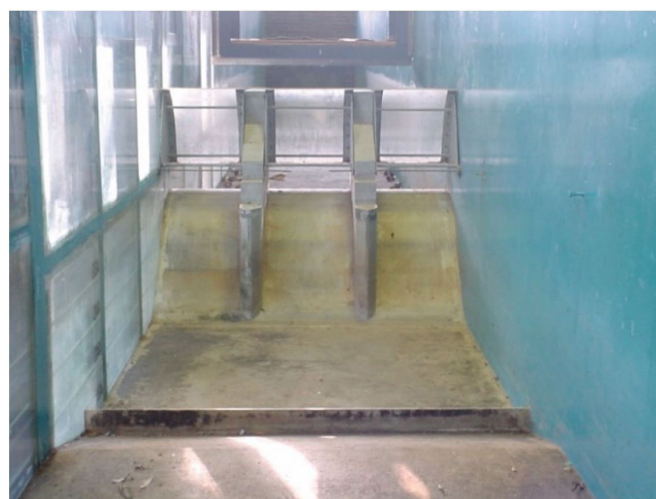
Figure 4. Spillway, stilling basin and end-sill (Wiest, 2008).
