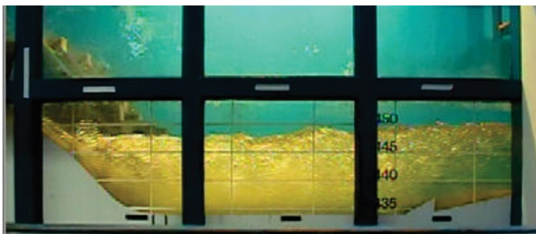
Figure 5. Hydraulic jump formed for Q_p = 4,000 \text{ m}^3/\text{s} and S = 1.61 (Wiest, 2008).
