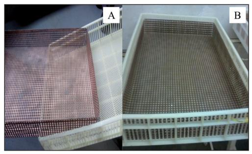
Figure 1. A- Copper hatch basket prototype developed for the experiment: fitted apart. B- Prototype attached to the conventional polypropylene hatch basket.
