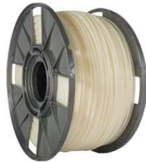
Figure 9: ABS filament used for printing on FDM printers. ABS filament (Frisotec®, São Paulo, Brazil)
