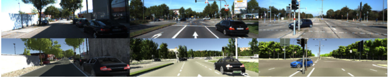
Figure 2.9: Examples from the virtual KITTI dataset compared with counterparts in the KITTI dataset.
