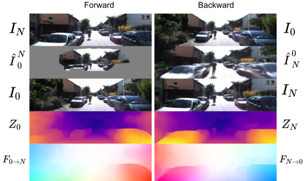
Figure 5.1: Example results from my method on the KITTI self-driving dataset. The first row shows the source image. The second row illustrates the projection of the source image into the target image. The third row shows the target image. The fourth row illustrates the estimated depth map, and the last row illustrates the estimated optical flow.
