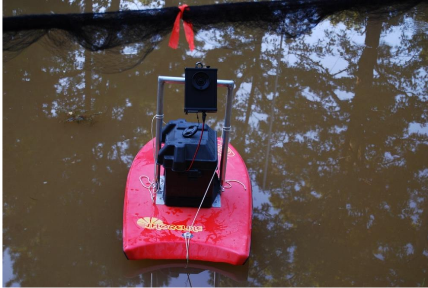
Figure 2.2 Acoustic lure deployed on a modified boogie board.
