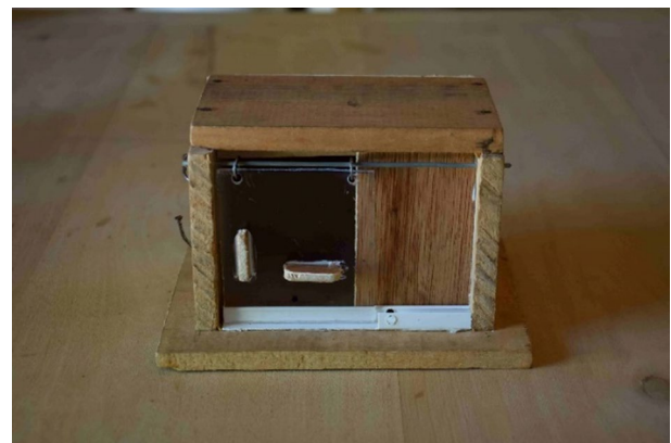
Fig. 1 Two-option foraging apparatus used to assess social learning. The door can be opened by either sliding or pulling
