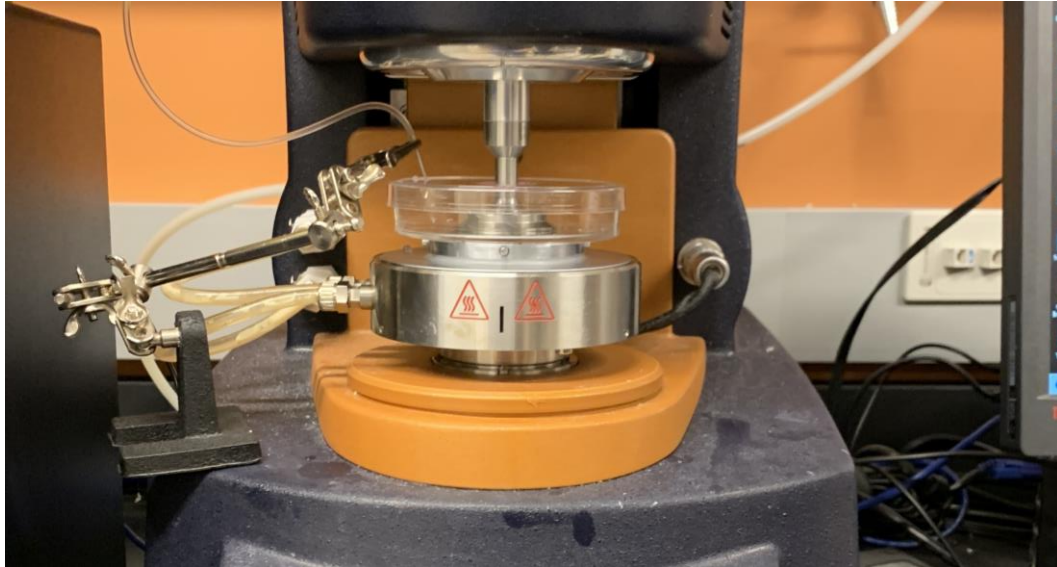
Figure H1. Rheometer setup used for the study of the impact of disturbed flow on protein expression
