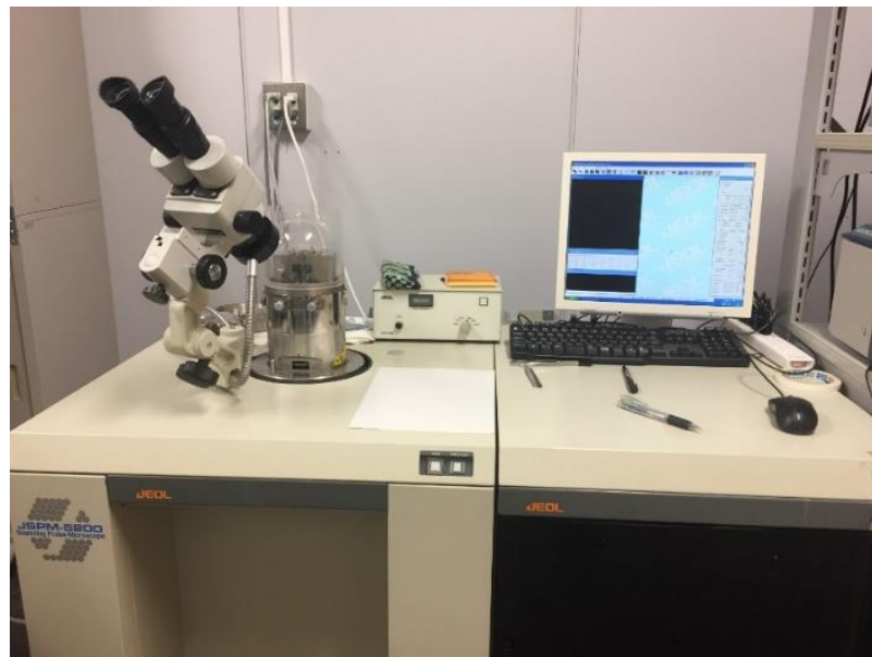
Figure 2.6. AFM system Jeol-SPM 5200
