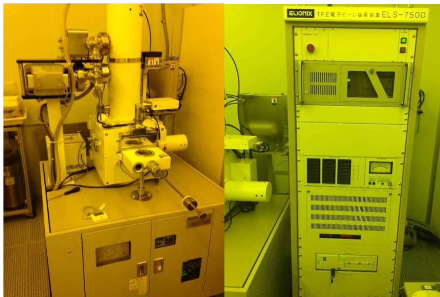
Figure 2.2. EB-lithography system model Elionix ELS-7500
