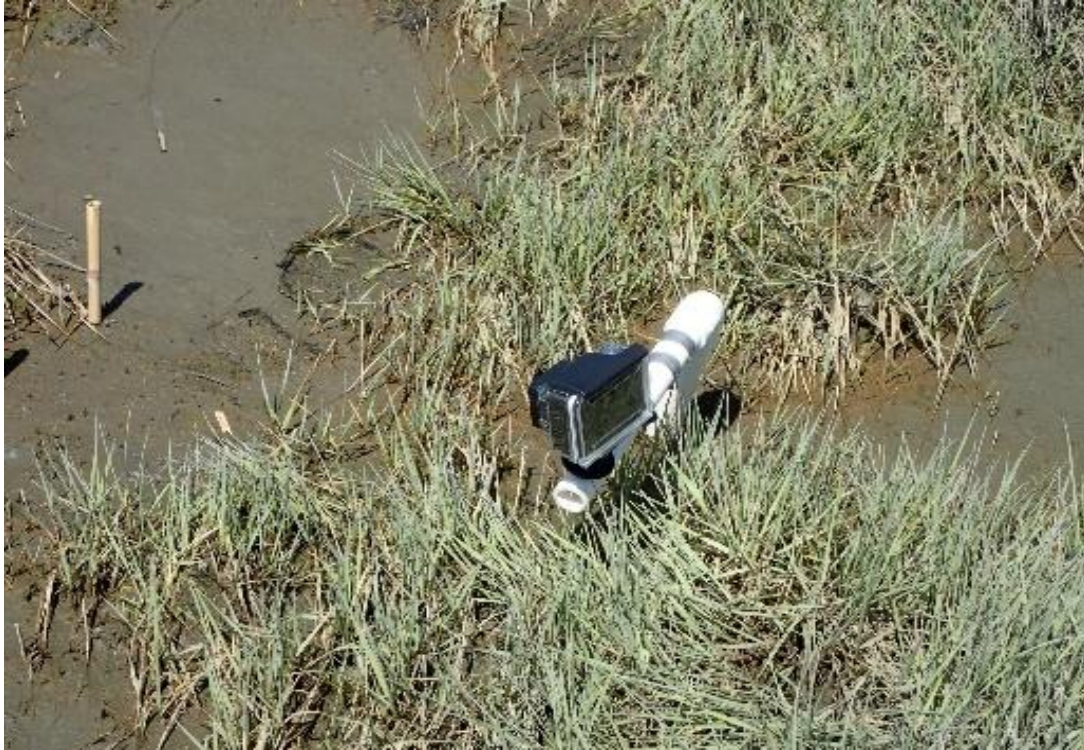
Figure 6. Go-Pro ® connected to a PVC pole that is in salt marsh sediments.
