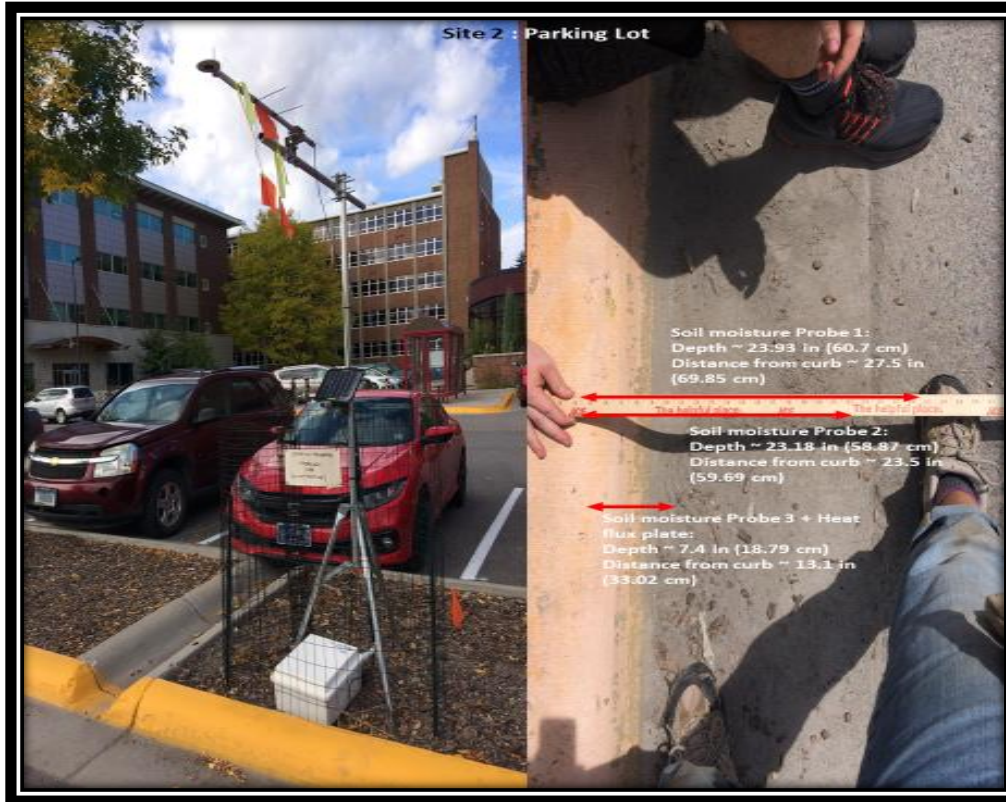
Figure C2. Site 2 instrumentation in the parking lot behind Skaggs Building at University of Montana. A trench was dug extending from the island with trees to under the asphalt and concrete lot. A soil moisture probe and one ground heat flux plate were installed at this location under the parking lot. The thickness of parking lot asphalt surface at this location is ~ 4.5 inches (11.43 cm).
