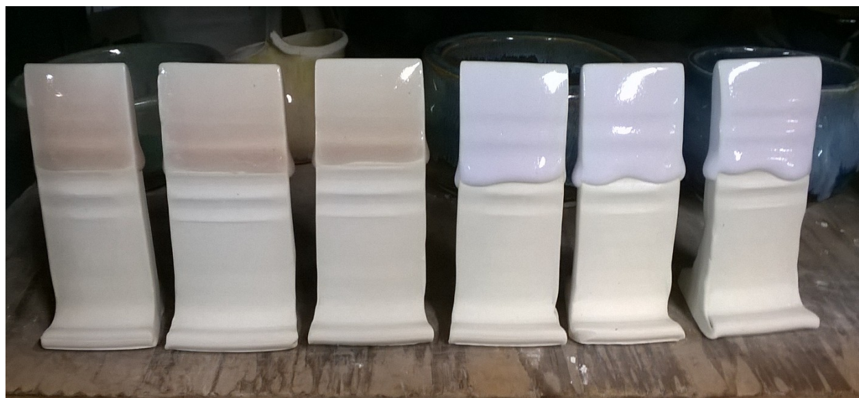
Figure S2. Oxidation-fired gold nanoparticle oxidation tiles. From left to right, 0.015, 0.050, and 0.100 % (wt/wt) Au without tin oxide and 0.015, 0.050, and 0.100 % (wt/wt) Au with 4% tin oxide.
