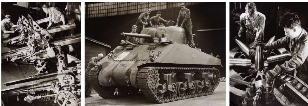
L to R: Pullman workers assemble field gun chassis; put final touches on a M4 Sherman tank; and test and finish artillery shells, probably all at the Pullman Michigan city plant. Source: Torkel Korling photographs, nos. A-22, A-33, and A-3, Tenneco Collection, acc. 593708.
