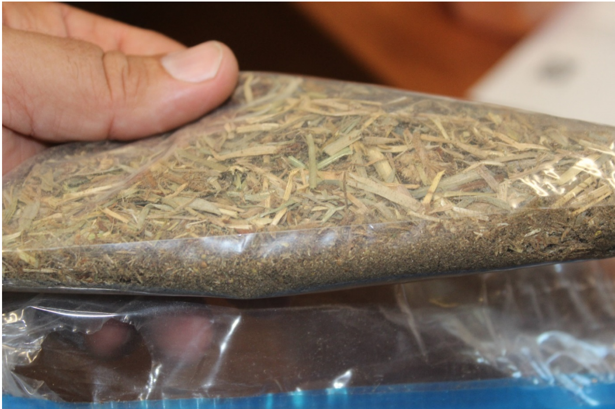
Figure 4. Never subdivide a sample before submitting it to the lab. Core samples are made up of both large and small particles that can segregate making it difficult to get a representative subsample. In this photo the fine particles have move to the bottom of the bag.
