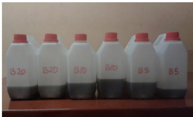
Fig. 3. Bio-oil/diesel emulsions three months after production.
