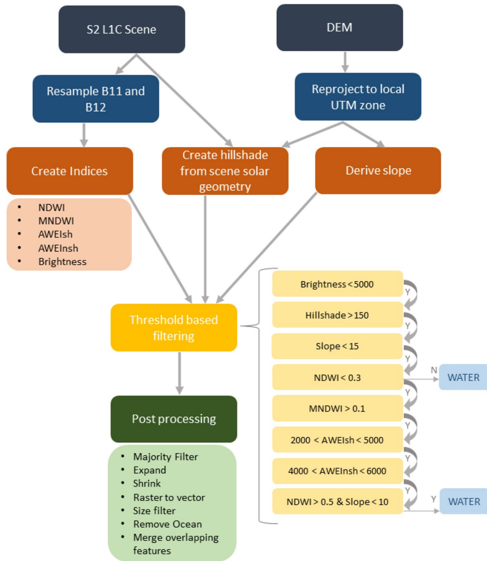
Figure 6. Flow diagram presenting the processing chain for classifying ice marginal lakes from Sentinel-2 imagery, including terrain indices generation using a DEM and multi-spectral indices thresholding, which is compiled through a decision tree classifier to extract water bodies.
