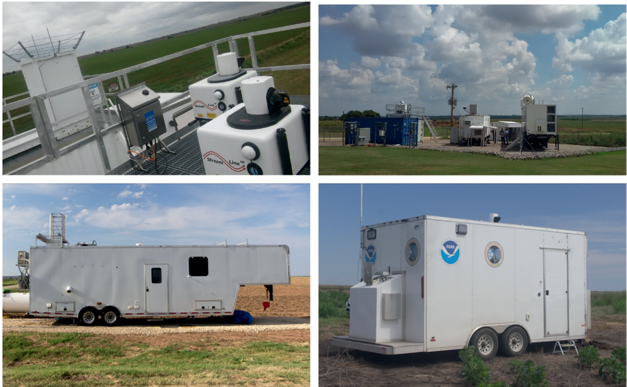
FIG. 5. Key scanning lidar systems operated during LAFE. (top left) DLIDs operated in vertically staring or six-point scanning pointing modes collocated with the SRLID. (top right) Collocation of (left to right) the NOAA DLID, the URLID, and the UDIAL at the SGP central facility all pointing northeast. (bottom left) The SPARC and (bottom right) the CLAMPS systems deployed and operated close to the SGP central facility.
