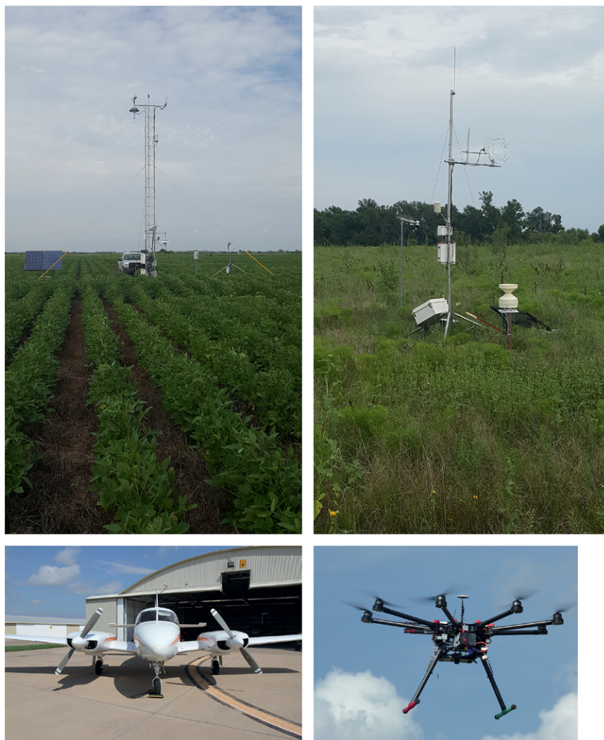
FIG. 6. In situ and airborne instruments operated during LAFE. (top left) NOAA ATDD and (top right) UHOH SEB towers over soybeans and natural vegetation mix. (bottom left) The Piper Navajo at Ponca City airport. (bottom right) NOAA ATDD sUAS operating close to the SGP central facility.
