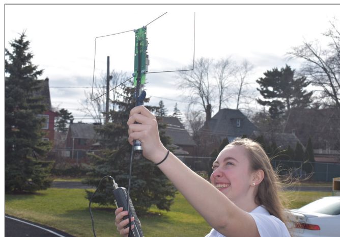
Fig. 2. An RDF in action. A student uses the “HANDI-Finder” to pinpoint the direction of a weather station. These finders work best in wide open, flat spaces.
