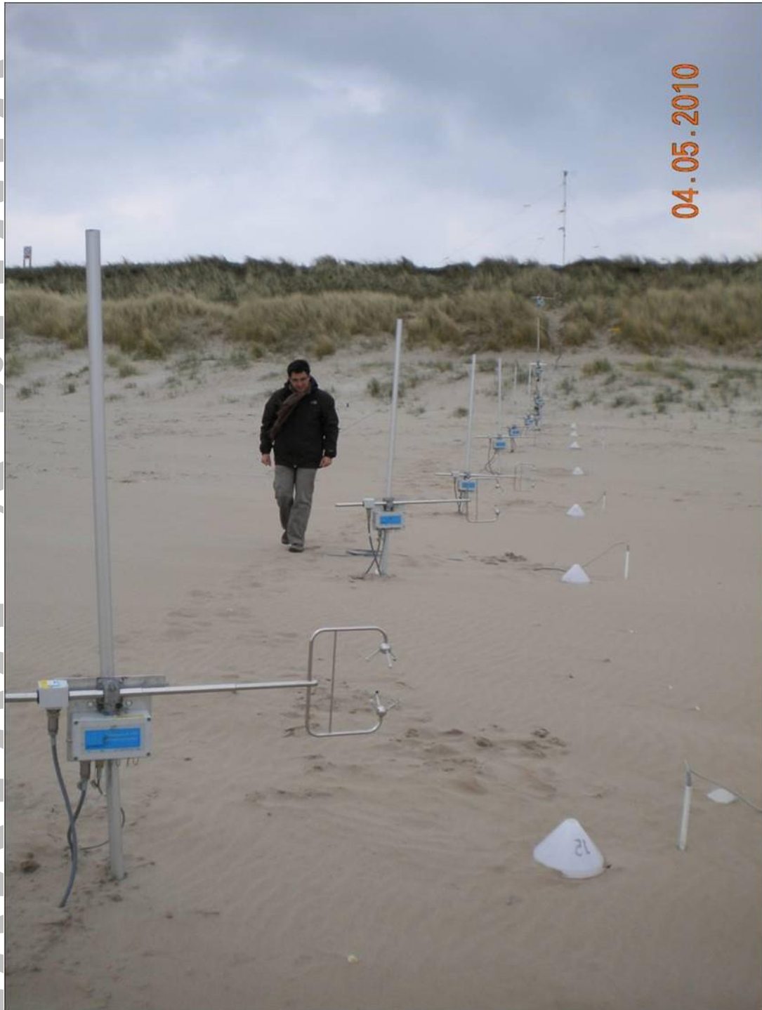
Figure 3: view of measurement stations along row B, looking landward. Forefront shows sonic anemometer mounted at 0.5 m above the ground and buried sand trap indicated by inverted funnel (trap inactive at time of picture taken).
