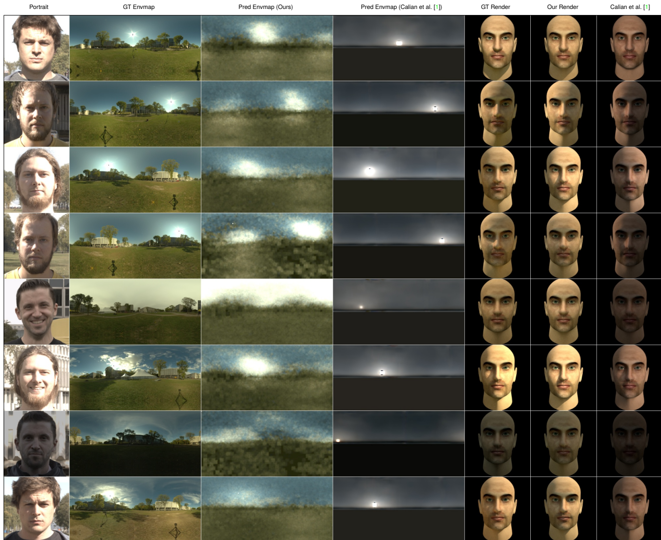
Figure 11. Results on 8 real faces from the Laval Face+Lighting HDR dataset and comparison with predictions from Calian et al. [1]. Left to right : input portrait image, GT environment map, predicted environment map with our method and Calian et al. 's, synthetic face rendered with GT environment map and with predicted environment maps.
