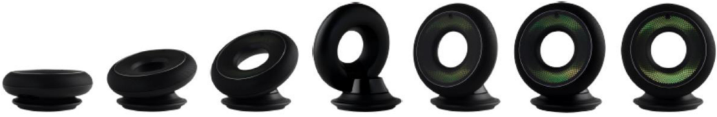
Fig. 5. Olly movement and positioning cues. Olly robot in different positions from idle and “unresponsive” (on left) to “up and highly attentive” (on right). Olly can “look” directly at the user (on right) versus show slightly averted gaze (third and fourth images from right), depending on the persona.
