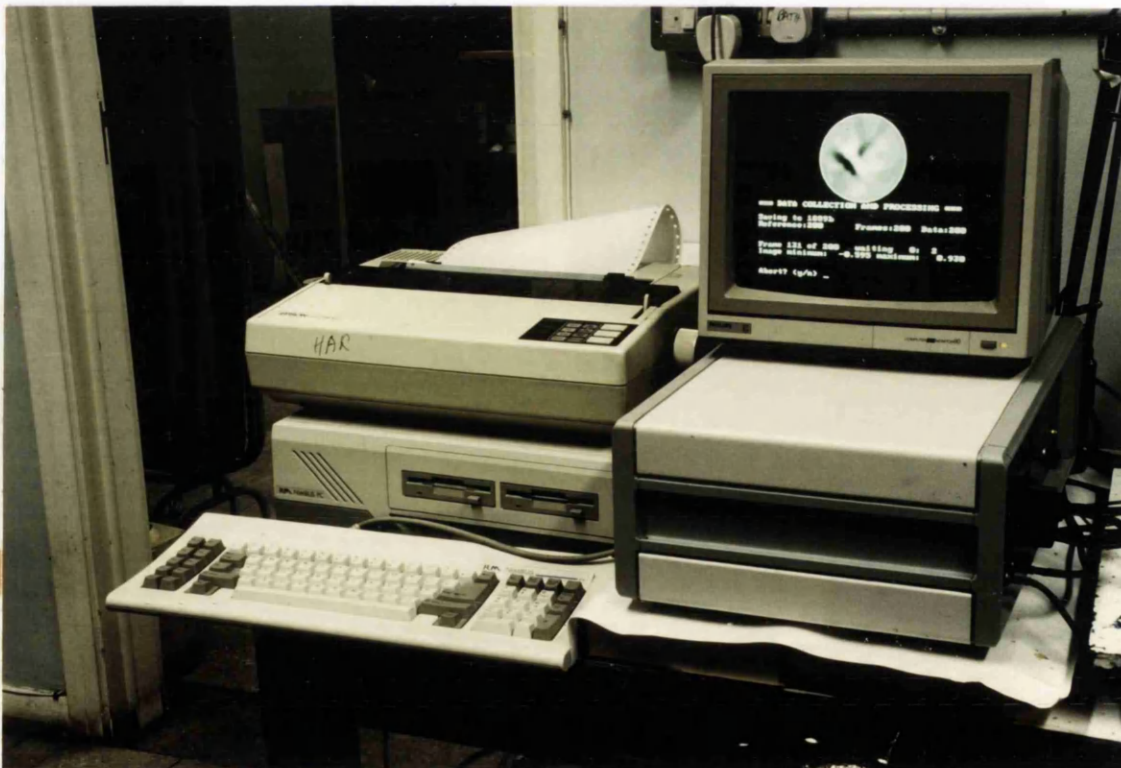
Figure 2.7. Physical dimensions of the Sheffield EIT system. The EIT hardware is housed in the box underneath the monitor. The other equipment is an IBM compatible computer and colour dot-matrix printer.
