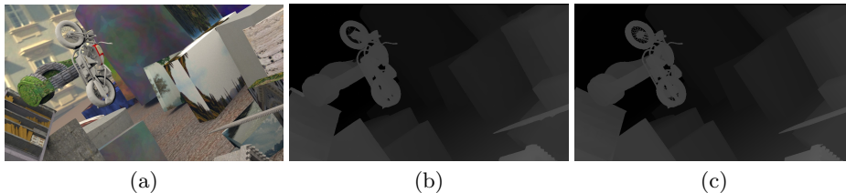
Fig. 2. Scene Flow test set qualitative results. (a) left stereo input image; (b) disparity prediction; (c) ground truth.
