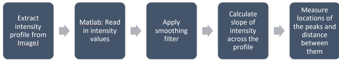
Figure 3.4: Semi-automated measurement vessel thickness measurement pathway
