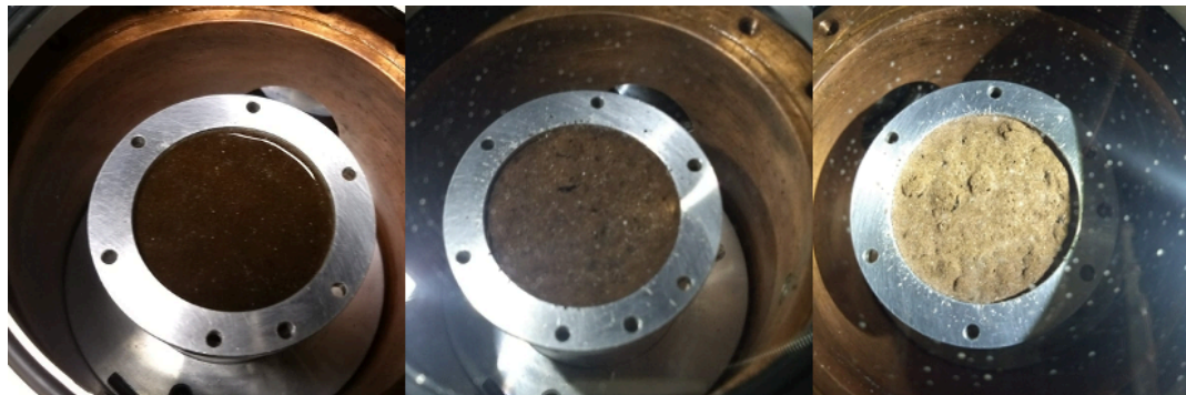
Figure 5.10: Samples of MgCl_2 \cdot 6H_2O with 1% PAH mix with 70% JSC Mars-1 at various stages of drying. Left is saturated with water, middle still slightly damp, right completely dry with hard crust formed
