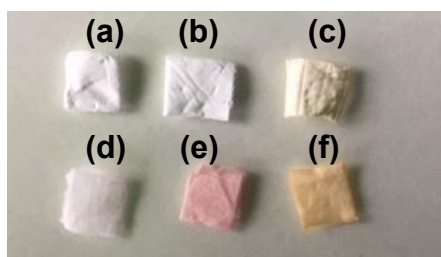
Figure 3-13: Digital photograph of electrospun fibres before and after incubation in BSA solution. Top row shows PCL patches before incubation (a,b,c), while the bottom row images were captured after 11 hours in BSA solution (d,e,f). Left – PFPA-untreated, UV-treated fibres (a,d), middle – PFPA-NHS before UV (b,e), right – PFPA-NHS after UV (c,f).
