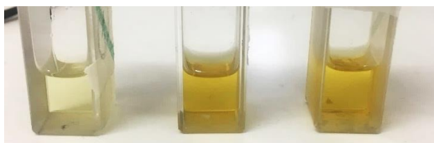
Figure 3-3: Digital photograph of the PCL-PFPA reaction products before purification. Three ratios of PCL to PFPA were tested: 9:1 w/w (left), 5:5 w/w (middle) and 1:9 w/w (right).
