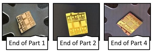
Figure 4.3: Device Fabrication Results
