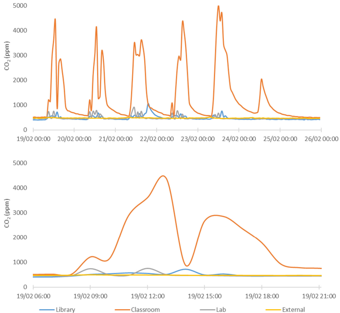
Figure 5.12: CO 2 levels in school spaces during a typical week (above) and typical day (below)
