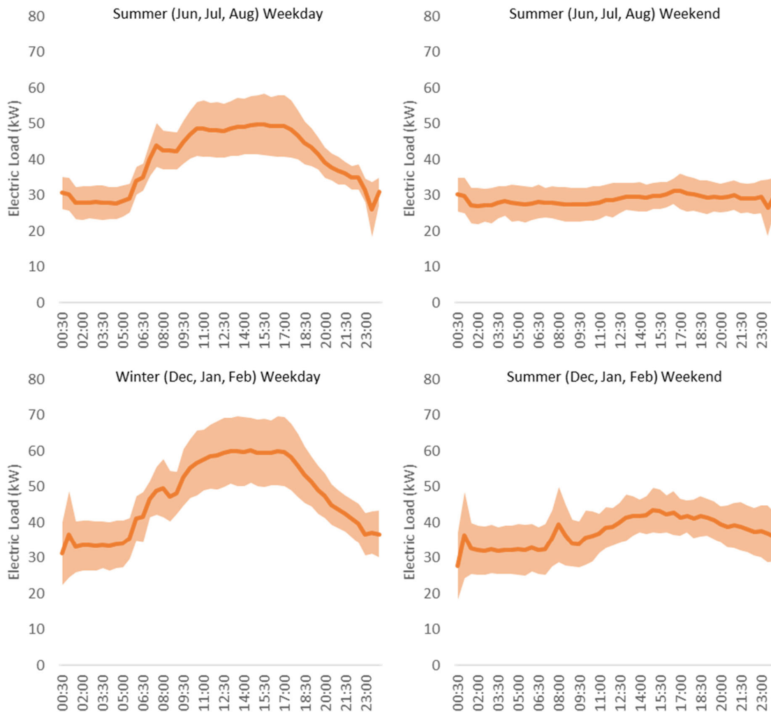
Figure 5.26: Average electrical demand and its standard deviation, for summer and winter months
