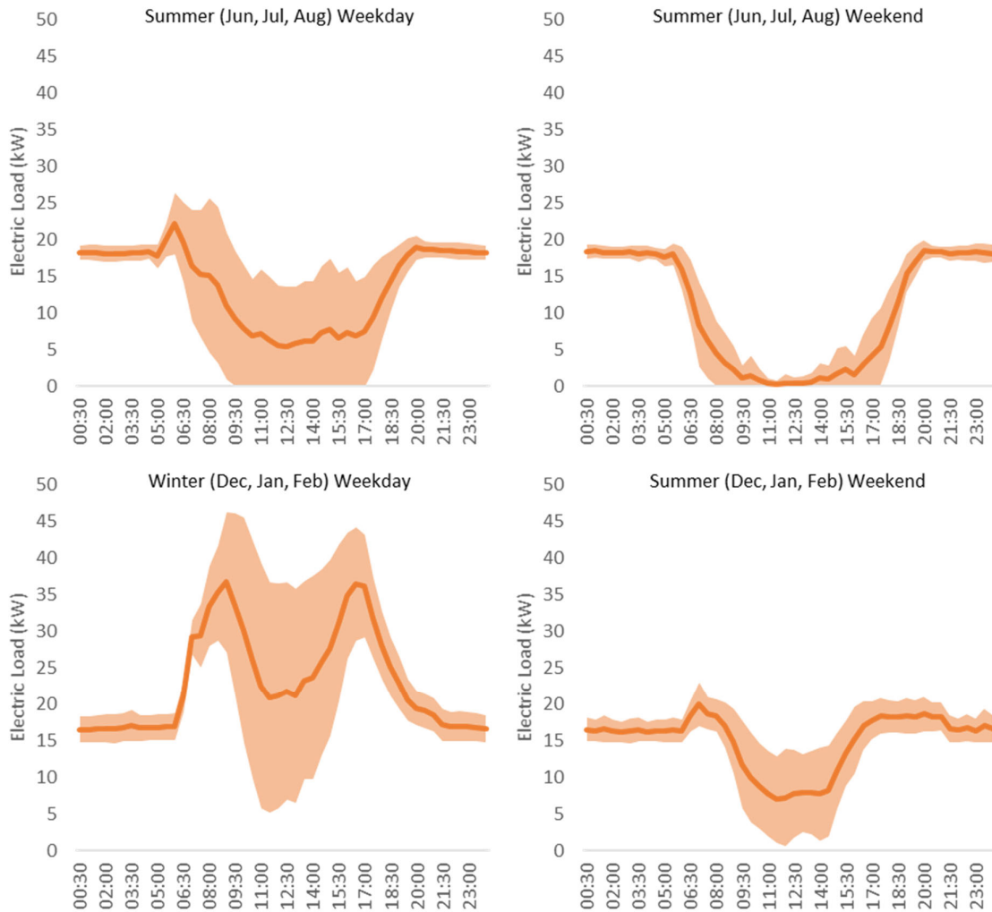
Figure 5.3: Average electrical demand and its standard deviation for the office building, for summer and winter months
