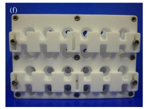
**Figure 3.12.** Bespoke Micro-24 feed delivery device Versions 1, 2 and 4. (a) and (b) Version 1: Single aluminium plate fabricated by BPR, GSK. (c), (d) and (e) Version 2: Three-plate aluminium device fixed with stainless steel screws. (f) and (g) Version 4: Two-plate PTFE device with two clamps that hold up to 12 feed lines each. Dimensions of Version 4 are indicated in Appendix B, Figures B.2-B.4.
