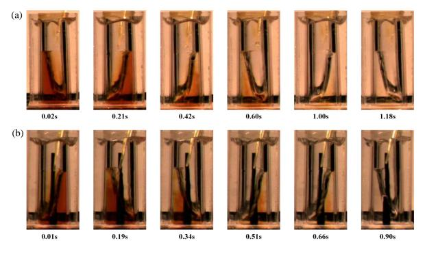
**Figure 5.4.** Representative high speed video images during Micro-24 mixing time experiments using the iodine discoloration method for: (a) REG cassette design and (b) PRC cassette design. Conditions for all experiments: dynamic start; 4mL fill volume; 800rpm shaking frequency;  $d_o$  5mm; 30°C. The experiments were performed as described in Section 2.8.2 and images were acquired using a DVR Fastcam (Photron, California, USA).
