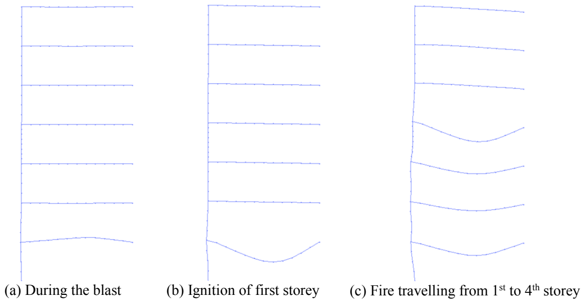
Figure 5.11. Deformation of the frame during the vertically travelling fire for an initial blast at the 1 st storey (5x magnification).
