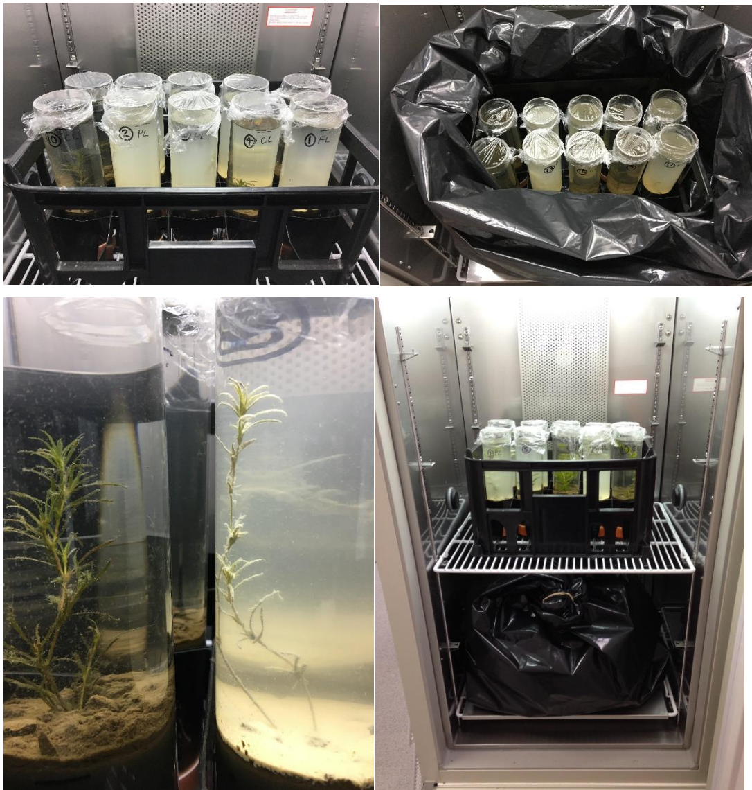
Figure 4.1. Control and LMB treated cores for Najas flexilis (bottom left), light treatment (top left) and dark treatment (top right) placed inside the incubator (bottom right) (© Kate Waters-Hart).
