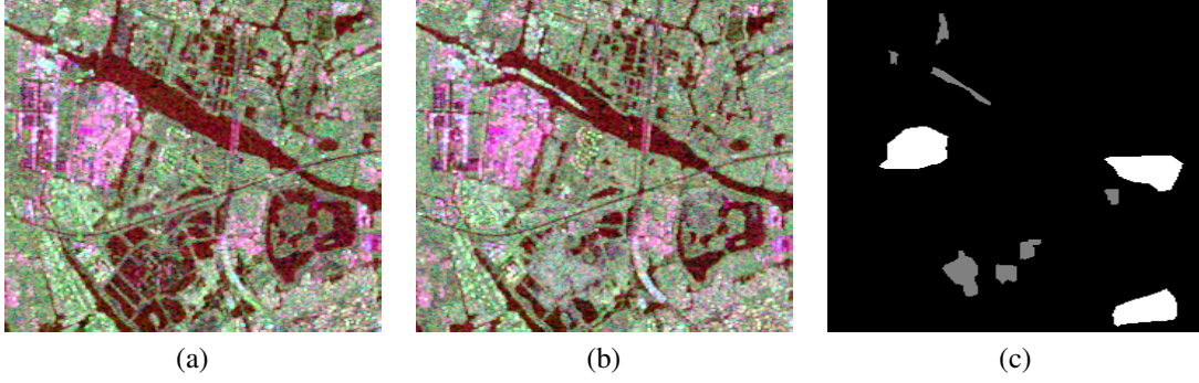
Fig. 5. Pauli RGB ( R = HH-VV , G = HV , B = HH+VV ) of quadpol RADARSAT-2 images captured over Suzhou city, East China on (a) April 9, 2009 and on (b) June 15, 2010, multilooked with 24-looks. (c) Truth change map; The white color means no-change, the color gray means change and the color black means unlabeled pixels.
