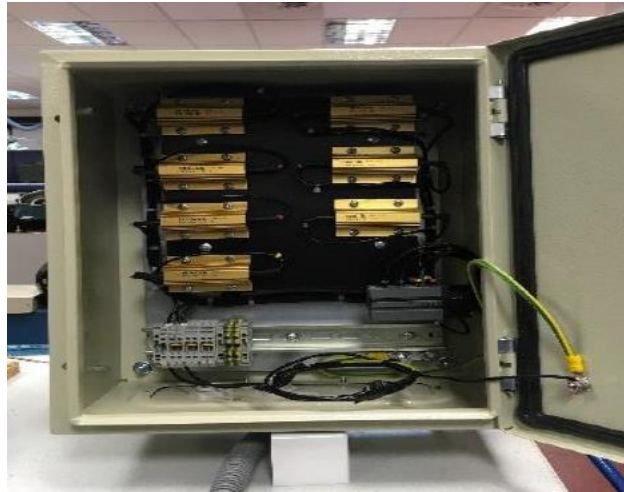
Figure 6-11 External resistor bank
