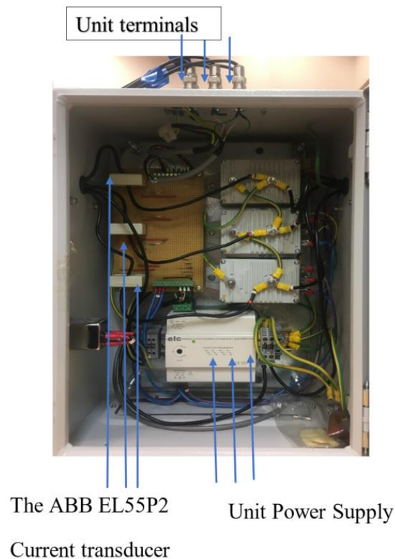
Figure 6-7 Photograph of the unit for three phase current measurements
