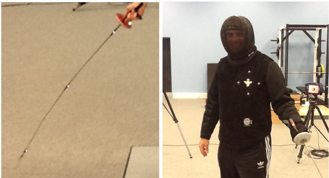
Figure 3.1. Marker placement on the foil (left), demonstrating three markers placed on the blade (5 cm from the base, middle, and 5 cm from the sword tip) and the target (right) four markers 15 x 15 cm apart on the fencing coach, with a central point to direct accuracy.
