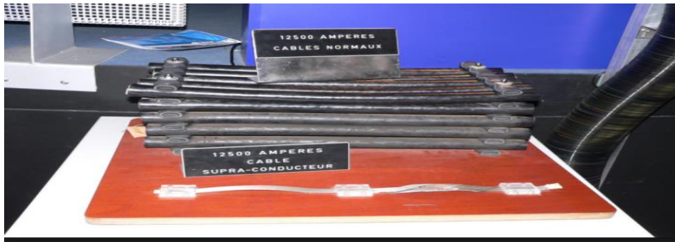
Figure 2.19: Comparison between the size of 12.5 kA conventional cable and superconducting cable [CERN-Cables]
