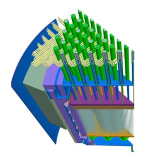
Figure 1: The geometry of a nuclear reactor core representing a physical domain D, on to which the different cross-sectional values of  $\sigma_{s}, \sigma_{f}, \pi_{s}, \pi_{f}$  are mapped, also as a function of neutron velocity.
