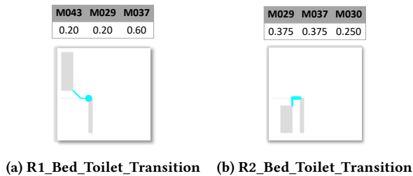
Figure 7: Examples of the ‘Bed Toilet Transition’ activity on R1 and R2: their sensor features and VLAIR images. ‘Bed Toilet Transition’ activates sensors ranging from bedroom to bathroom, which results in a rich spatial pattern visible in the encoded VLAIR images.
