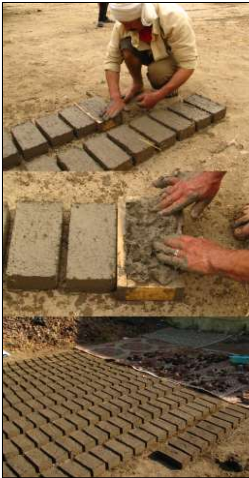
Figure 5: Experimental brick forming and drying (photographs by authors).
