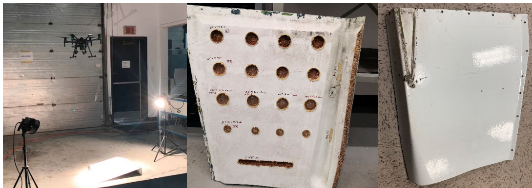
Figure 3. Second experimental setup (left), underside defects (middle), non-defective side (right).
