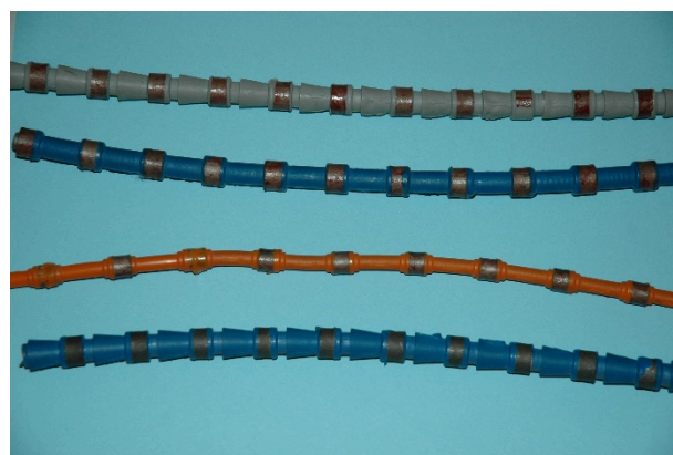
Figure 16. Examples of polycrystalline diamond wires, in the figure there are various diamond wire saws which are characterized by the number of wire beads (40–28 pcs/m) and the diameter of beads (11.5–6.3 mm).
