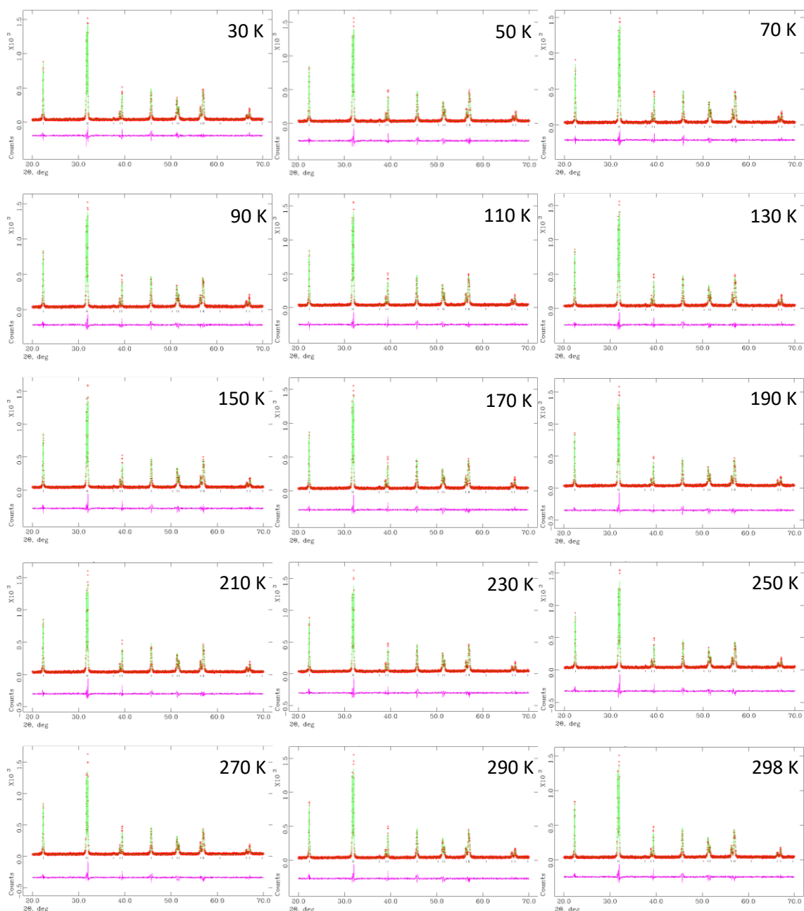
Figure A3.19: Rietveld refinements obtained from LT PXRD of \text{Bi}_{0.95}\text{Na}_{0.05}\text{Fe}_{0.95}\text{Nb}_{0.05}\text{O}_3 in the temperature ranges 30 K to 298 K.
