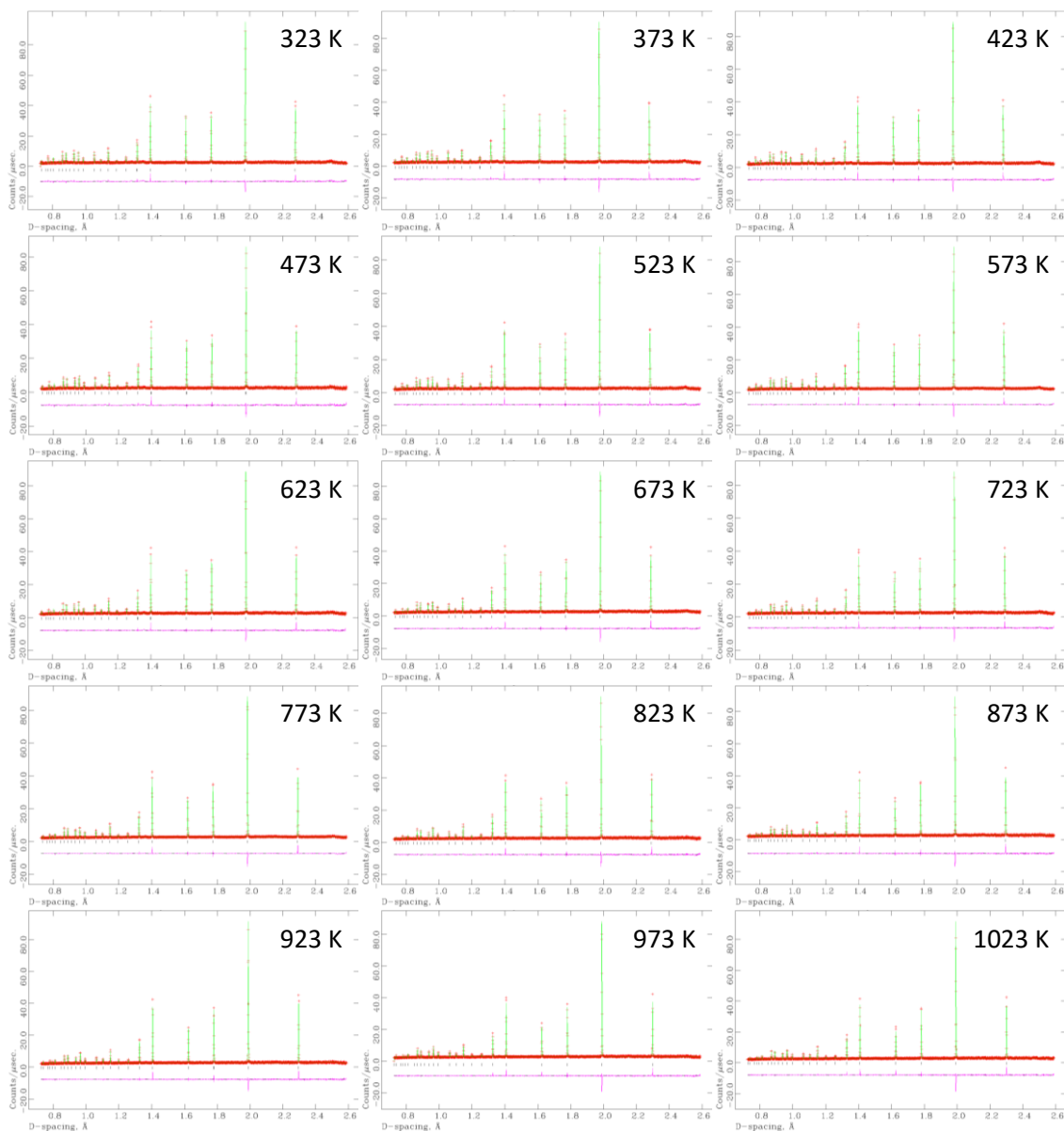
Figure A2.19: Rietveld refinements obtained from HT PND of \text{Bi}_{0.5}\text{Na}_{0.5}\text{Fe}_{0.5}\text{Nb}_{0.5}\text{O}_3 in the temperature range 323 K to 1023 K.
