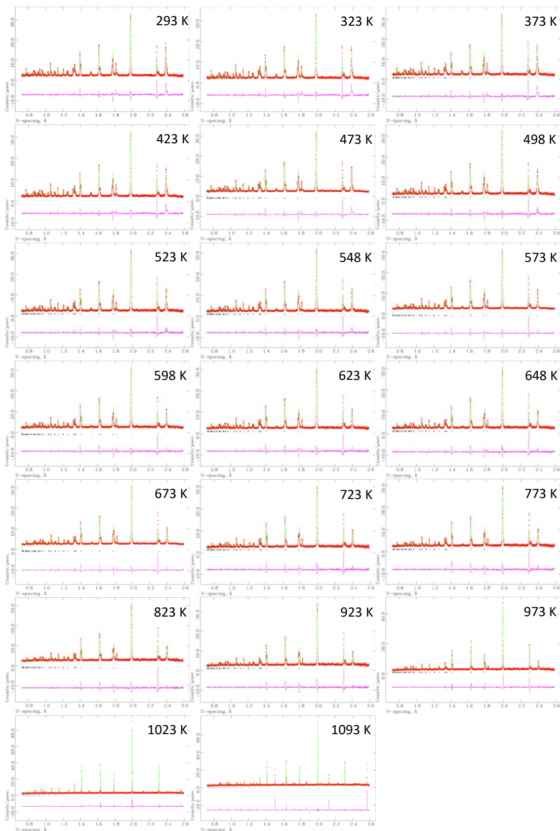
Figure A1.10: Rietveld refinements to R3c model obtained from HT PND of \text{Bi}_{0.9}\text{Na}_{0.1}\text{Fe}_{0.9}\text{Nb}_{0.1}\text{O}_3 in the temperature range 293 K to 1093 K.
