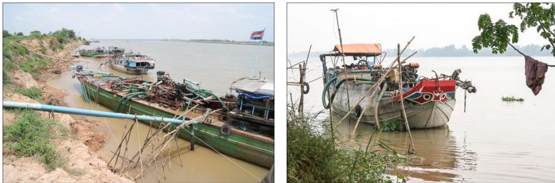
Figure 5-3: Sand mining 'pumping dredge' boats on the Mekong main stem in Cambodia (left) and Bassac in Cambodia (right) (Bravard et al, 2013).
