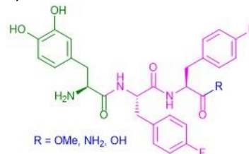
Figure 28. The chemical structure of the peptides of R-COOMe, R-CONH 2 , and R-COOH. Dopa is in green, the antifouling motif, fluorinated phenylalanine, in pink, and the different ending groups, in blue.
